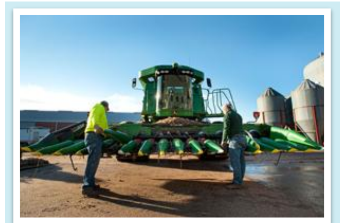
Farmers make adjustments to a harvest header for a quality corn harvest.
